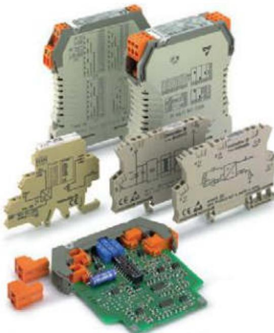
**2-way isolation** separates the signals from each other electrically and decouples the measuring circuits. Potential differences – caused by long line lengths and common reference points – are eliminated. Furthermore, the electrical separation protects against irreparable damage caused by overvoltages as well as inductive and capacitive interference.
