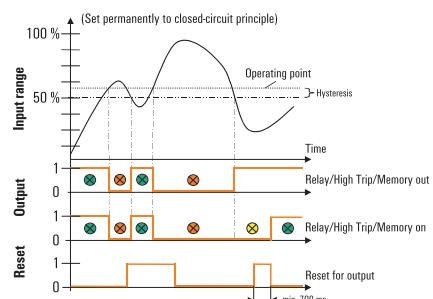
**Abb.2: Undervoltage monitoring**Alarm set to "low trip"
