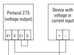
Calibration of a transmitter with four-wire connection and current or voltage input
