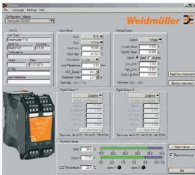
The free software TTA-Set allows fast and uncomplicated configuration of the WAVE TTA . Easily adjustable measurement window, transmit functions and switching thresholds, as well as different thresholds and alarms for faults.
