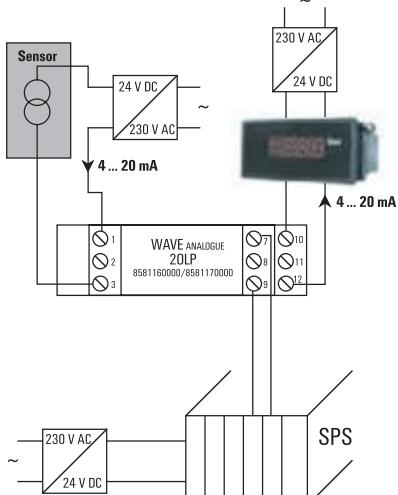
**Signal distributor****Supplied by current loop**
