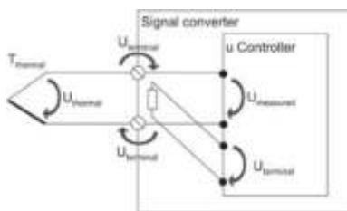
The microprocessor compares the value measured with the characteristic curve for the thermocouple in its memory and calculates the corresponding value on the "ideal characteristic curve". At the output, it supplies the latter to an amplifier, which produces the analogue value in linear form. The output stage converts this into a standardised value or into a switching output with a switching threshold.
