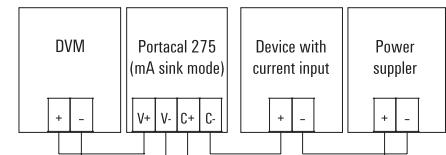
Calibration of a transmitter with two-wire connection
