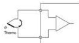
In order to compensate for the error to the measured value which arises here, the temperature is measured at the clamping terminal. The microprocessor in the signal converter reads the value measured there and calculates it against the measured value. This procedure is known as cold junction compensation.
