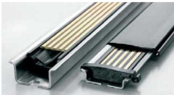
The resistant gold-plated contacts ensure a permanent and reliable contact. The ACT20M modules are simply snapped onto the mounting rail and are automatically in contact with the DIN rail bus.
