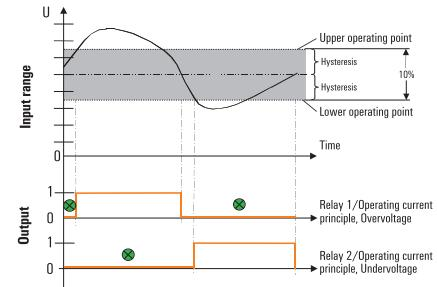
**Fig. 2: Overvoltage and undervoltage monitoring, example of setting**
